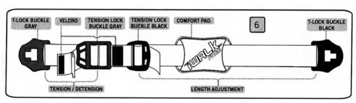
tensioning only (to put on and take off the crutch). Fully extend both sections of the Strap by lifting on the lip of the Tension Lock Buckles while pulling out on the T Lock Buckles. Repeat for all 3.
